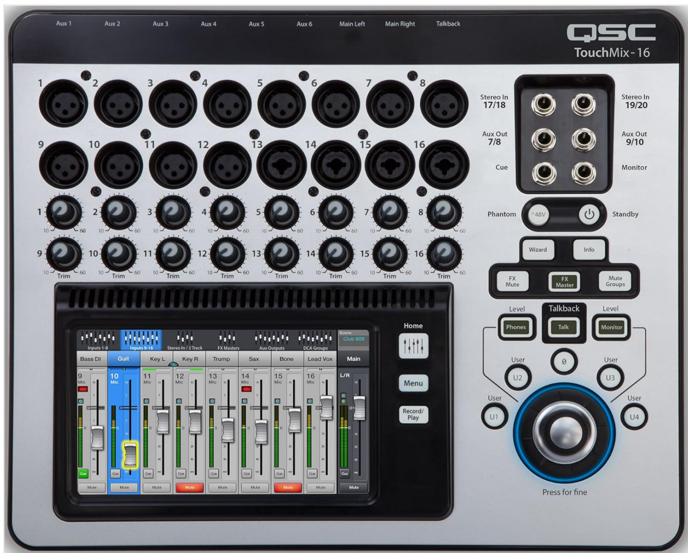
Top-down view of the QSC TouchMix-16, highlighting all input channels and control knobs.
