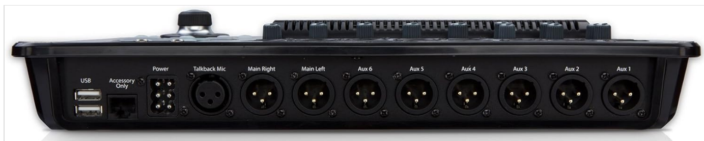
Rear view of the QSC TouchMix-16, showing various output ports including Aux, Main, and USB connections.
