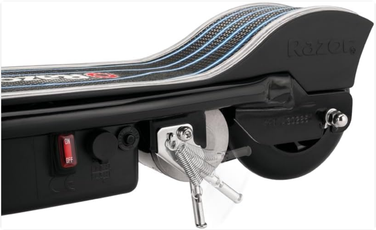
Figure 3: Location of the retractable kickstand, charging port, and power on/off switch on the scooter's deck.
