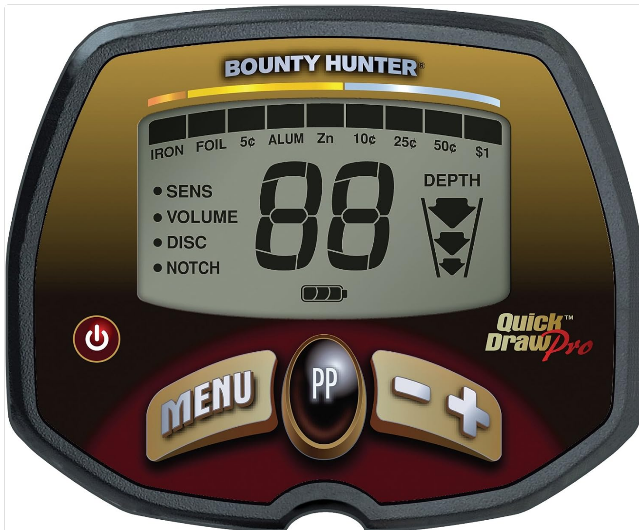
Figure 2: Close-up of the Quick Draw Pro control panel and LCD display.
