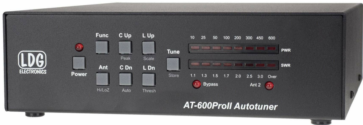
Image: Front panel of the LDG Electronics AT-600PROII Automatic Antenna Tuner, showing controls, LED bar graphs for PWR and SWR, and dimensions (10.5"L x 8.5"W x 2.5"H).
