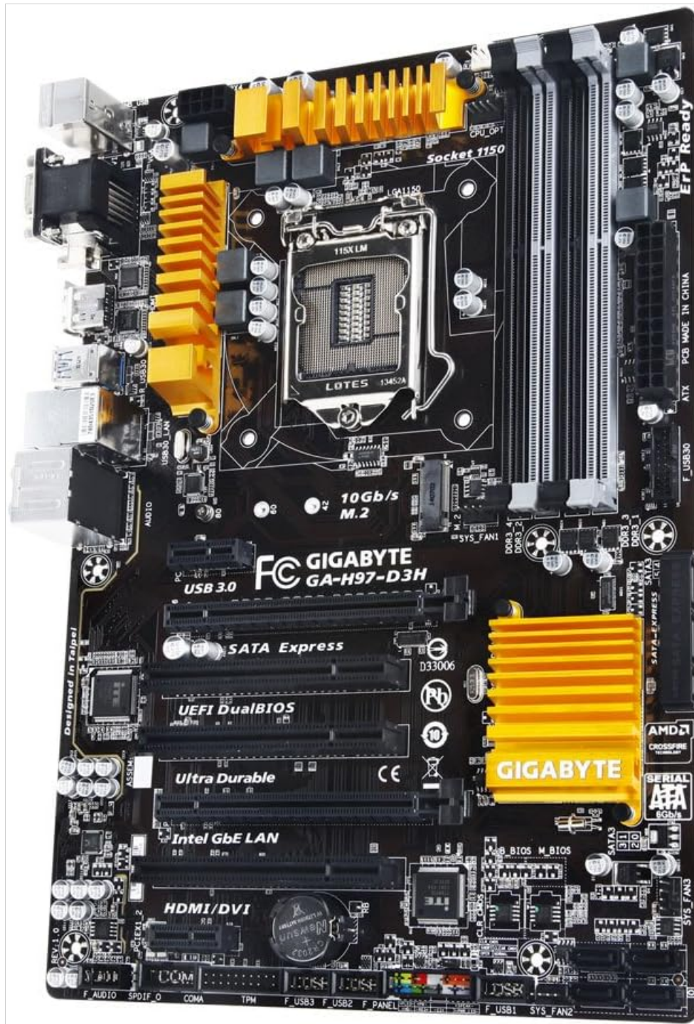
Figure 2: Angled view of the GIGABYTE GA-H97-D3H Motherboard. This perspective provides a clearer view of the CPU socket area, the golden heatsinks over the VRM and chipset, and the arrangement of the DDR3 memory slots.
