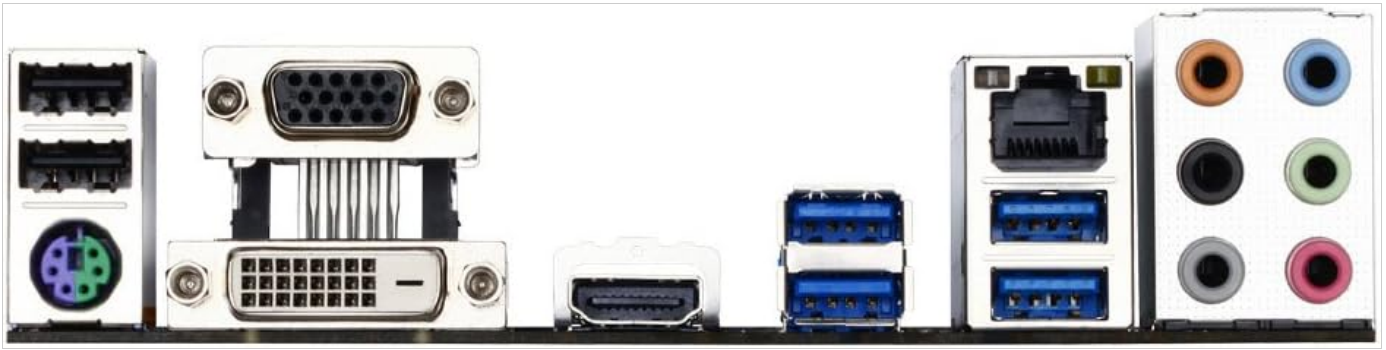
Figure 4: Rear I/O Panel Connectors. A detailed view of the rear input/output ports, including PS/2 keyboard/mouse, USB 2.0, USB 3.0, VGA, DVI, HDMI, Gigabit Ethernet, and 7.1 channel audio jacks.
