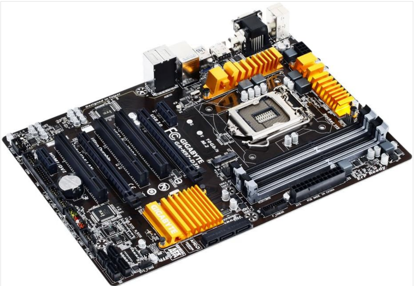
Figure 3: GIGABYTE GA-H97-D3H Motherboard Rear I/O. This image shows the various input/output ports available on the back panel, including USB ports, video outputs (VGA, DVI, HDMI), Ethernet, and audio jacks.
