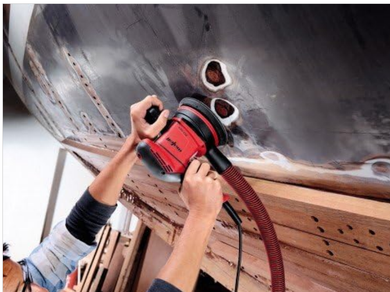
Image: The Mafell EVA 150 E sander being used on a wooden panel, showing the dust collection system attached and the smooth motion of the tool.
