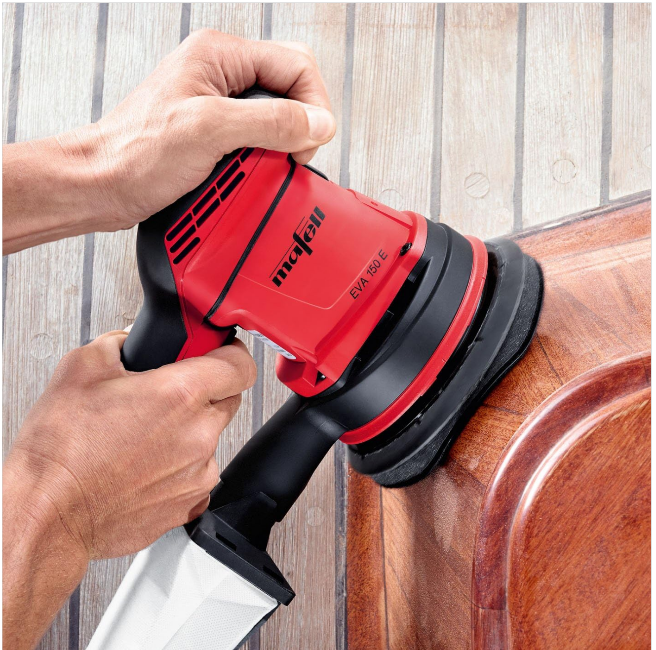
Image: The Mafell EVA 150 E sander being used on a wooden panel, showing the dust collection system attached and the smooth motion of the tool.
