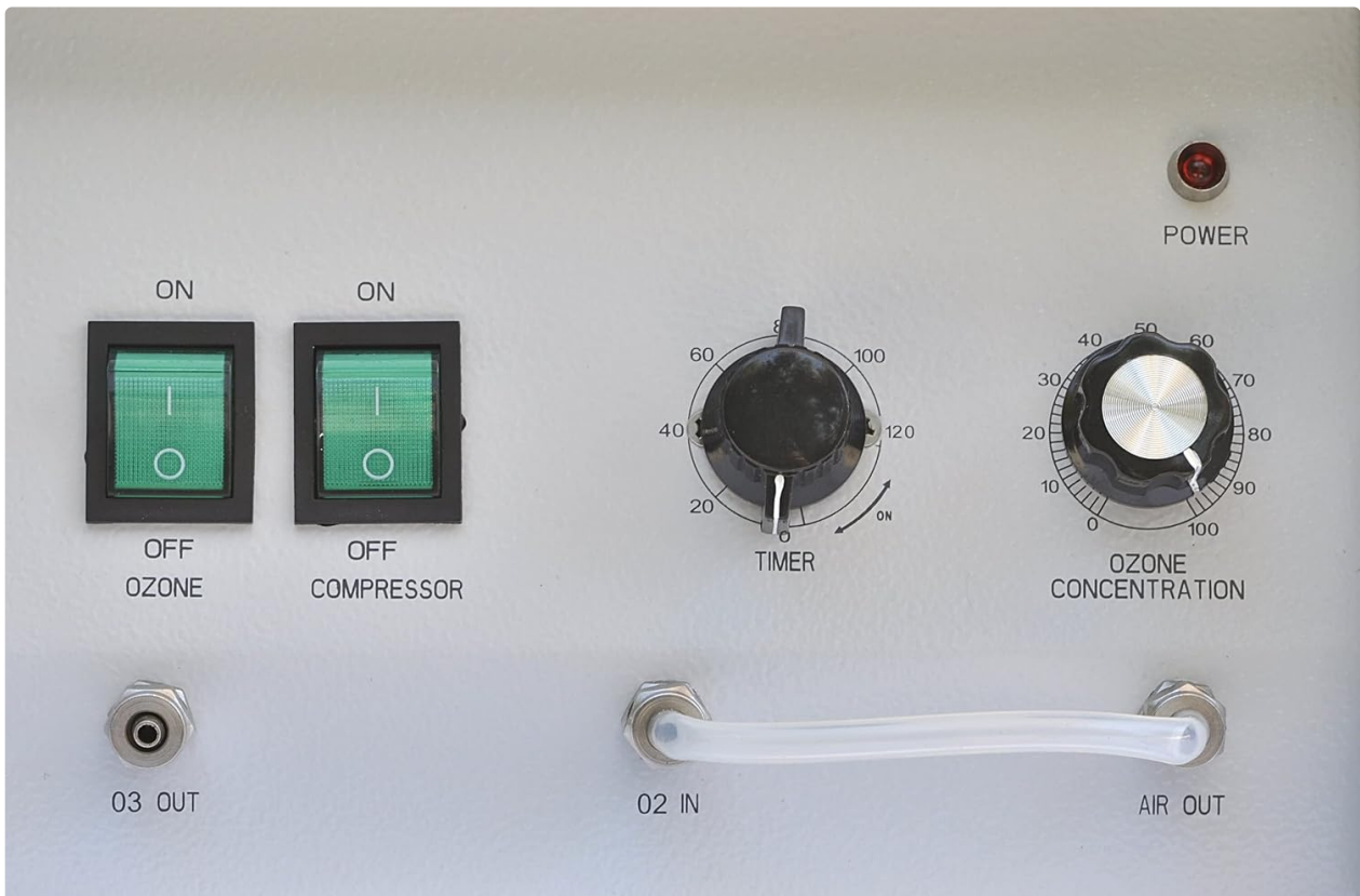
Image: A close-up of the control panel, highlighting the switches and dials for setting operation time and ozone output.
