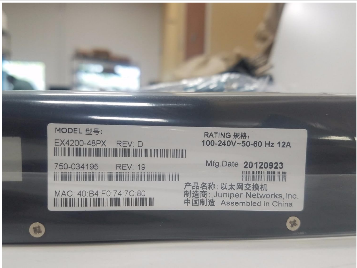
Figure 4.3: Product label displaying the Model: EX4200-48PX REV: D, Rating: 100-240V~50-60 Hz 12A. Key identifiers include the MAC address: 40:B4:F0:74:7C:80 , Part Number: 750-034195 REV: 19 , and Manufacturing Date: 20120923 . The device is manufactured by Juniper Networks, Inc. and assembled in China.
