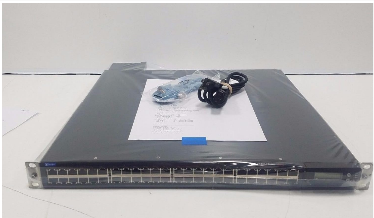
Figure 4.1: Front view of the Juniper EX4200-48PX switch, highlighting the 48 Gigabit Ethernet ports.
