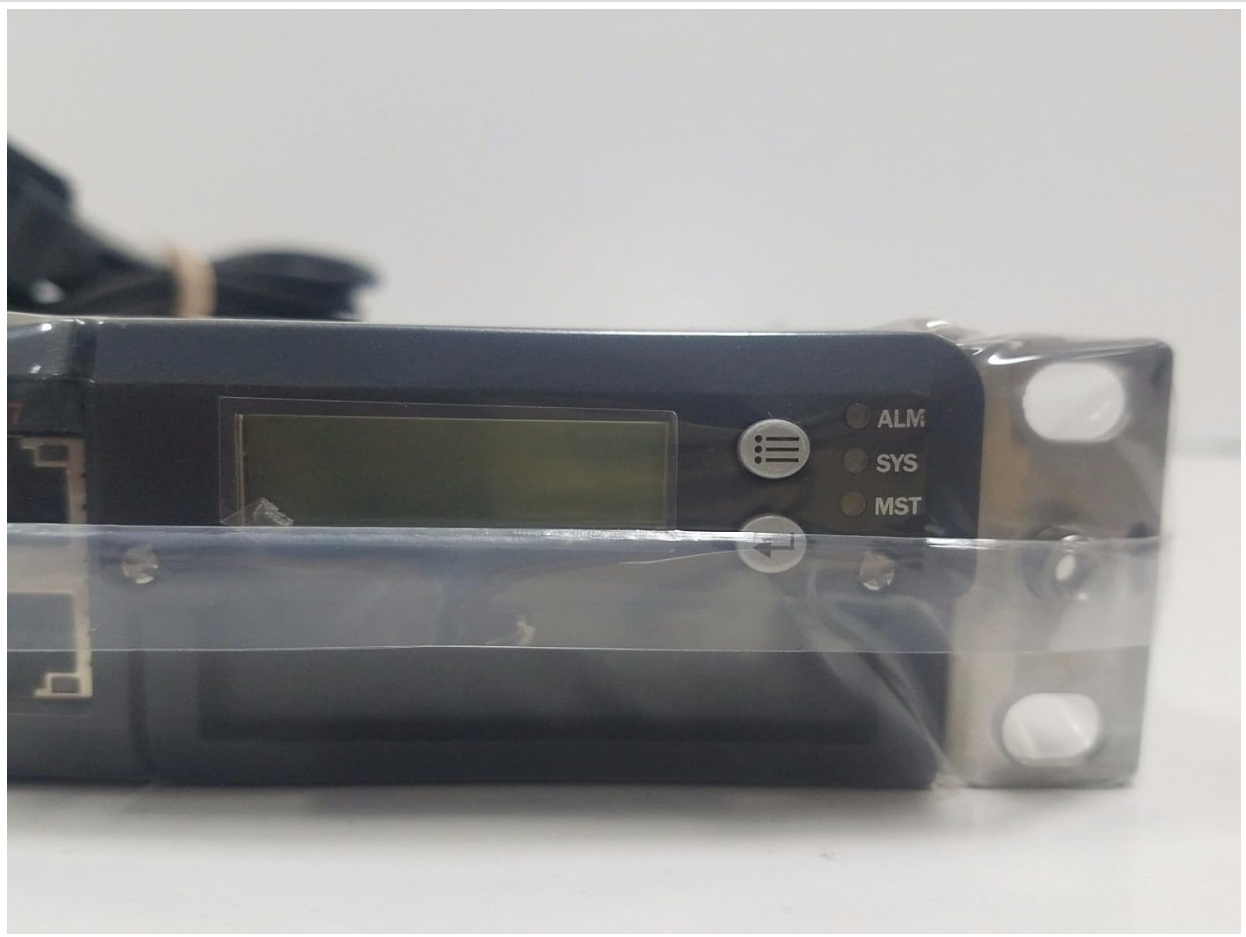
Figure 4.2: Detail of the front panel showing the LCD display and status indicators: ALM (Alarm), SYS (System), and MST (Master). These LEDs provide quick visual status of the device's operational state.
