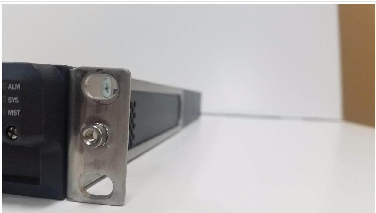
Figure 4.4: A close-up view of a rack mount ear, demonstrating the attachment point for securing the switch within a standard equipment rack.
