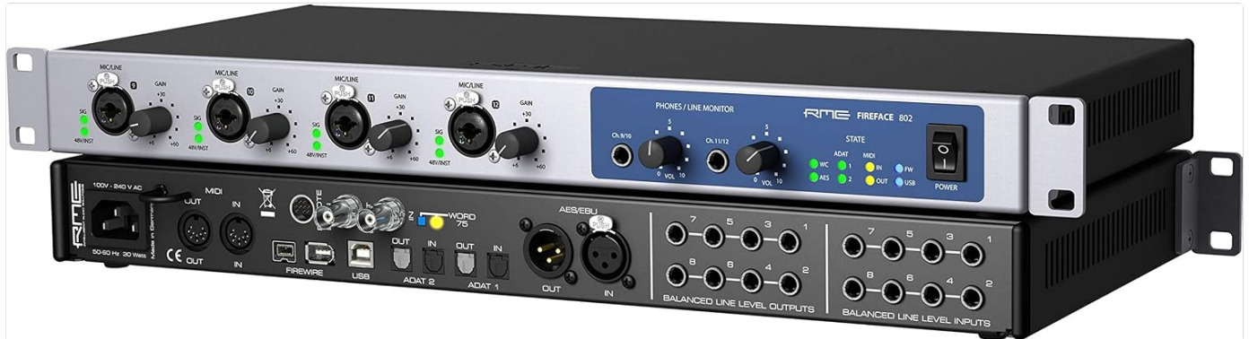
Figure 2: Detailed view of the RME Fireface 802. The top unit highlights the front panel controls including four mic/line gain knobs, 48V phantom power buttons, instrument (DI) buttons, and the Phones/Line Monitor section with volume controls and state indicators for ADAT, MIDI, USB, and FireWire activity.
