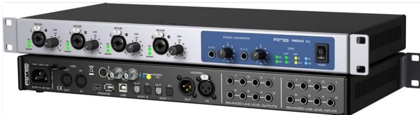
Figure 1: Front and rear view of the RME Fireface 802 audio interface. The top unit shows the front panel with four microphone/line inputs, gain controls, phantom power buttons, and monitor section. The bottom unit shows the rear panel with various analog and digital inputs/outputs, USB, FireWire, MIDI, and power connections.
