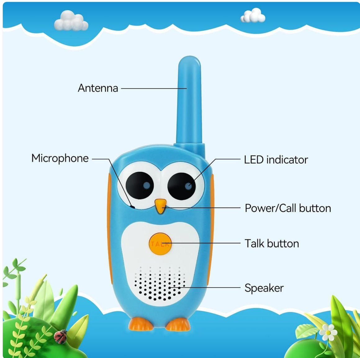
Image 2: Labeled components of the Retevis RT30 Walkie Talkie.
