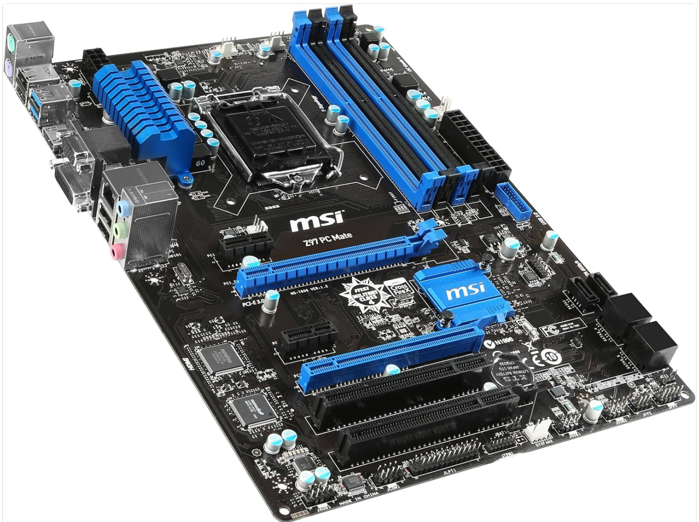
Figure 2: Angled view of the MSI Z97 PC Mate Motherboard. This perspective highlights the CPU socket area, RAM slots, and the heatsinks.
