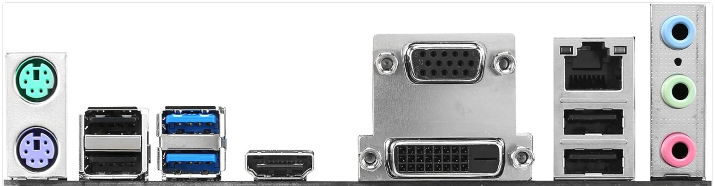
Figure 3: Rear I/O Panel. This image displays the various ports available on the back of the motherboard, including USB, Ethernet, audio jacks, and video outputs (VGA, DVI, HDMI).
