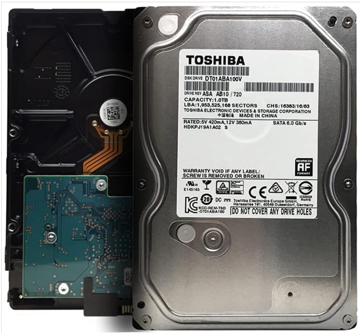
Figure 4.1: Top view showing the product label and bottom view revealing the PCB.
