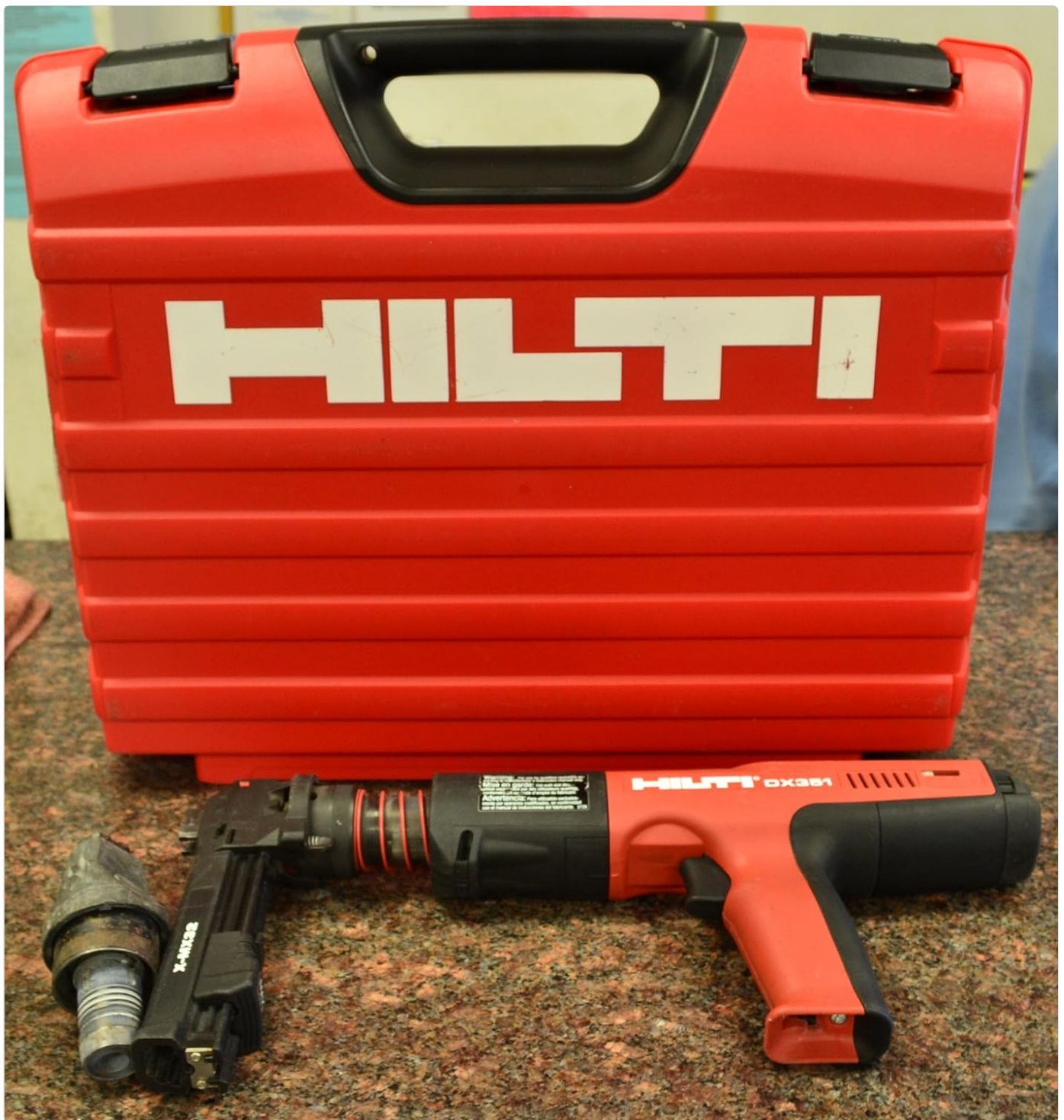
Figure 3.1: Hilti DX 351 Powder-Actuated Tool with X-MX 32 Magazine and its red carrying case. The image shows the red Hilti branded case at the top, and the red and black tool with the attached magazine lying in front of it on a speckled surface.
