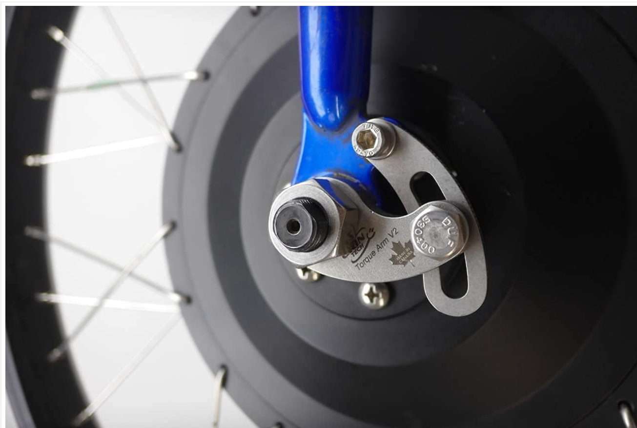
Figure 3: Installed Grin Technologies Torque Arm V2. This image provides a close-up view of the torque arm properly installed on a bicycle's front fork, securing the hub motor axle.
