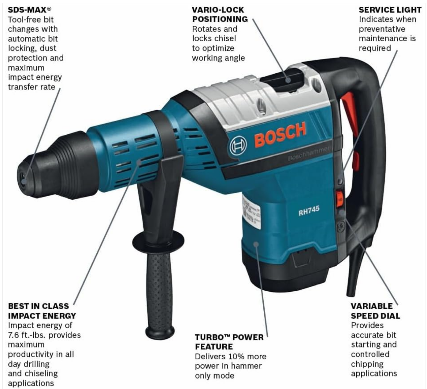
Figure 2: Detailed view of the Bosch RH745 Rotary Hammer with key features labeled.
