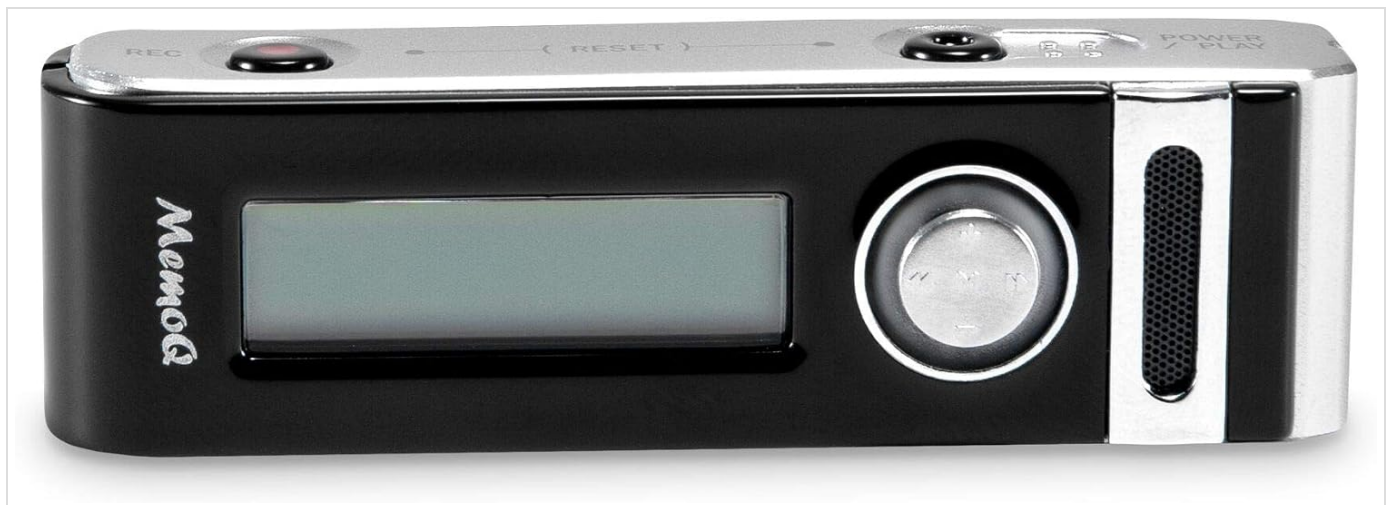
Figure 2: Front view of the MemoQ MR-740, highlighting the LCD display, navigation wheel, and integrated speaker grille.
