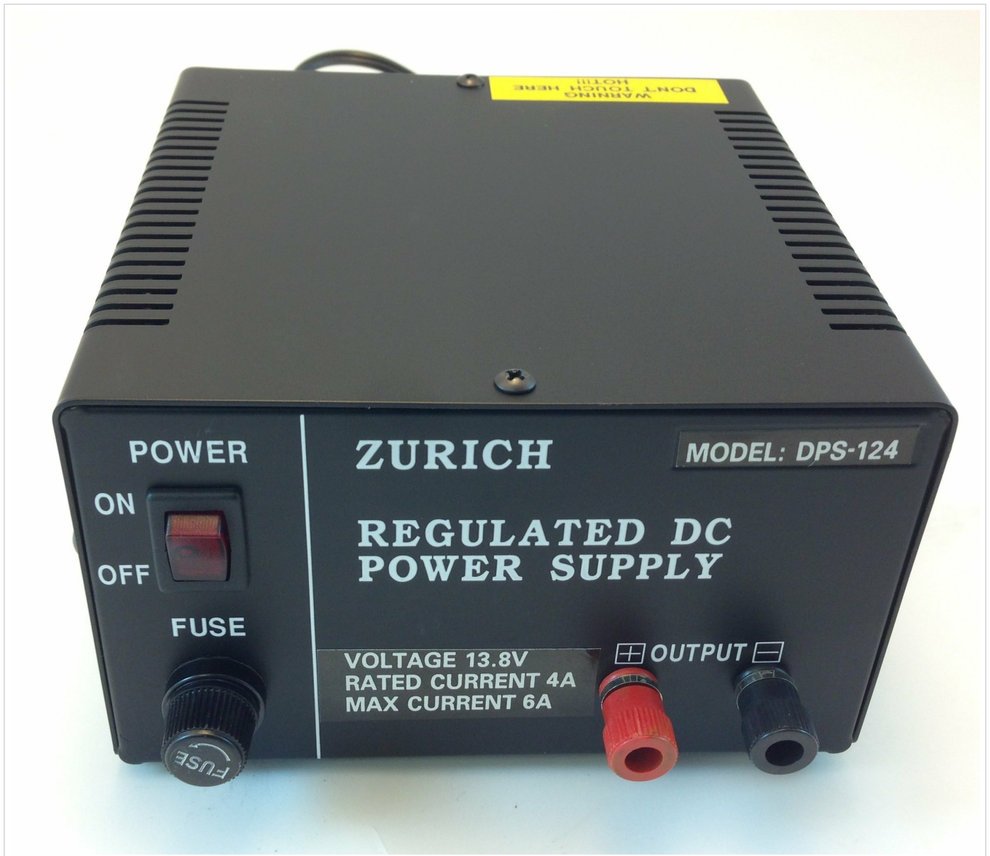
Figure 1: Front panel of the ZURICH 13.8V Regulated Power Supply. This image displays the power switch, fuse holder, positive (red) and negative (black) output terminals, and a label indicating the voltage (13.8V), rated current (4A), and maximum current (6A). The model number DPS-124 is also visible.
