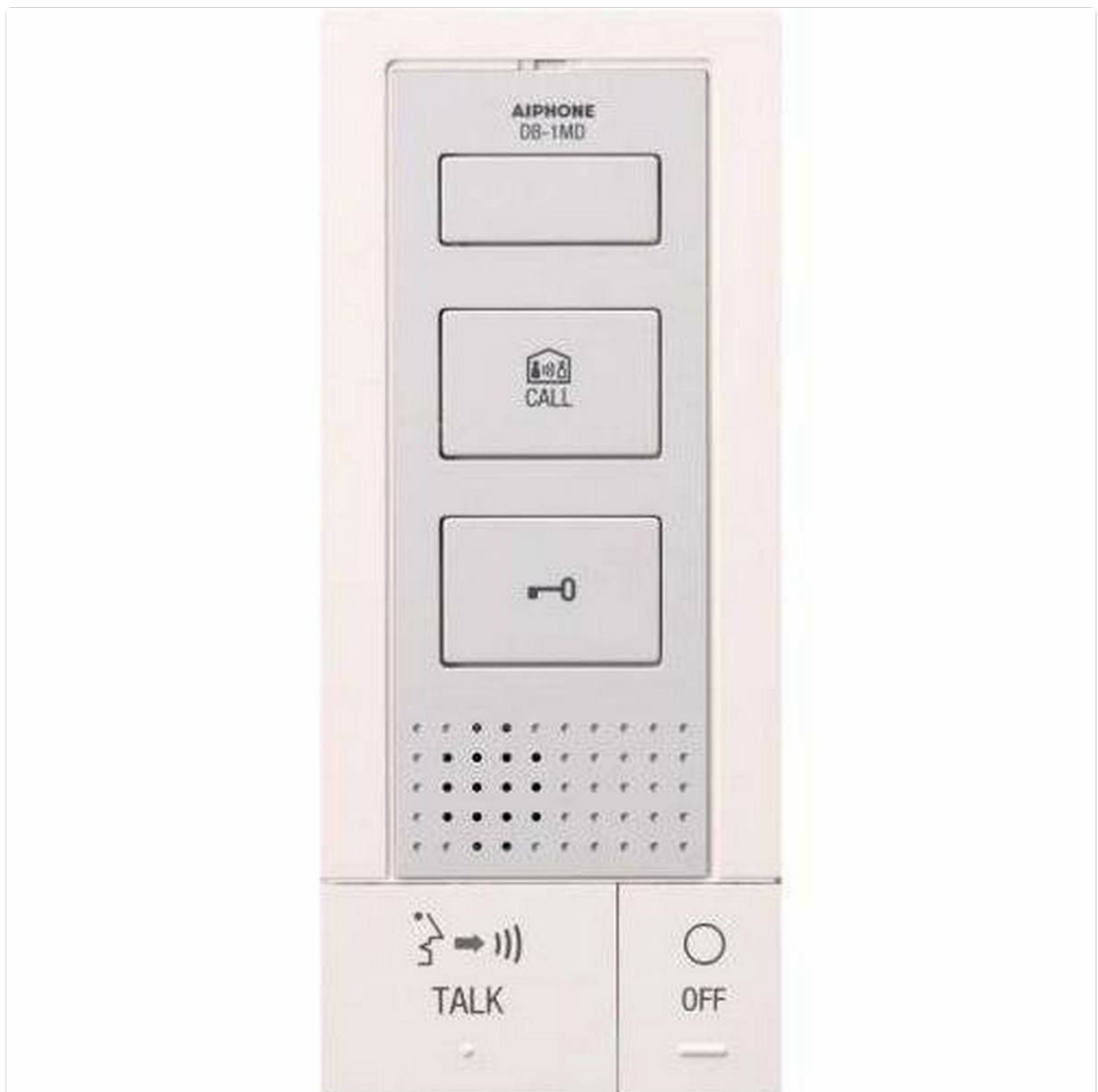
Figure 1: Front view of the Aiphone DB-1MD Tenant Master Station. The unit features a speaker grille at the bottom, a 'TALK' button on the left, and an 'OFF' button on the right. Above the speaker, there are three rectangular buttons: the top one is blank, the middle one has a 'CALL' icon (with a house symbol), and the bottom one has a key icon, which typically functions as a door release button. The model number 'AIPHONE DB-1MD' is visible at the top.
