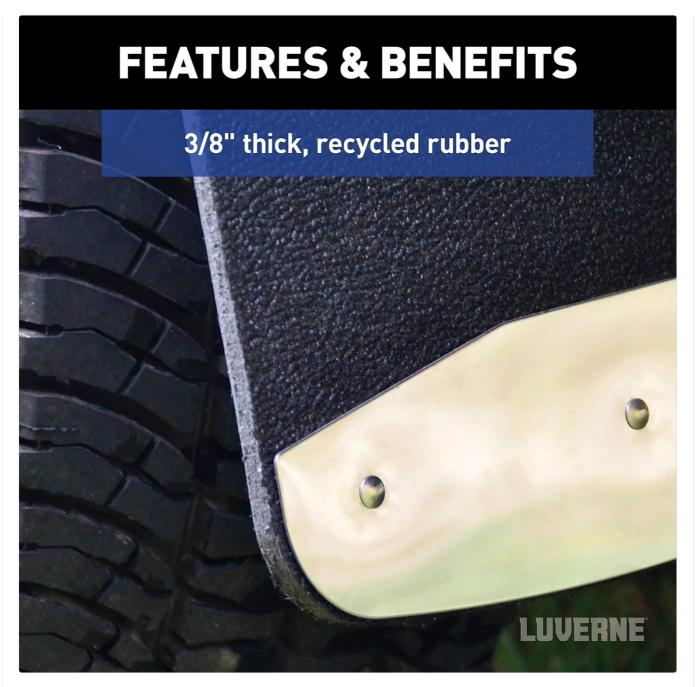
A detailed close-up shot of the mud guard's surface, emphasizing the 3/8-inch thick recycled rubber and its textured finish designed to hide minor scuffs.
