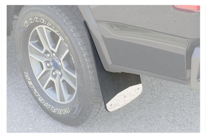
A close-up view of the polished 18-gauge stainless steel plate located at the base of the mud guard, designed to provide additional protection and a stylish accent.
