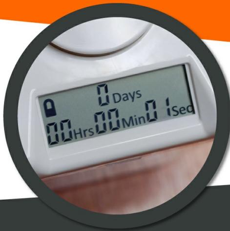
Figure 4: The display indicating the locked status and remaining time.
