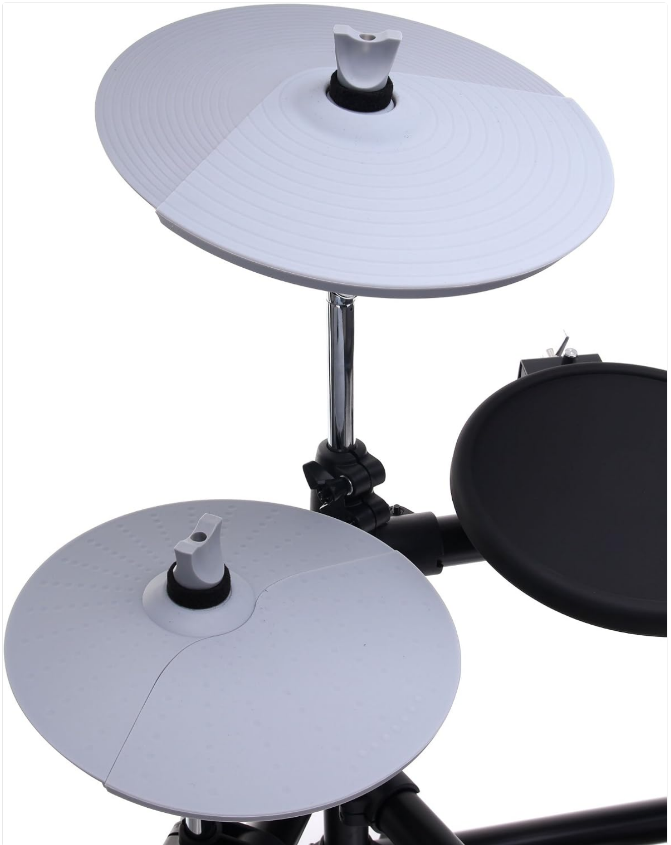
Figure 4.3: Two cymbal pads attached to the drum rack.
