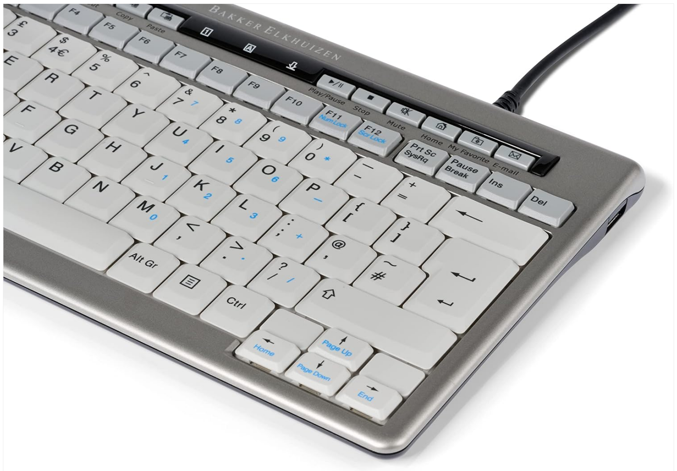
Image: Close-up of the top row of keys on the BakkerElkhuizen BNES840DUK keyboard, highlighting the function keys and integrated media controls.
