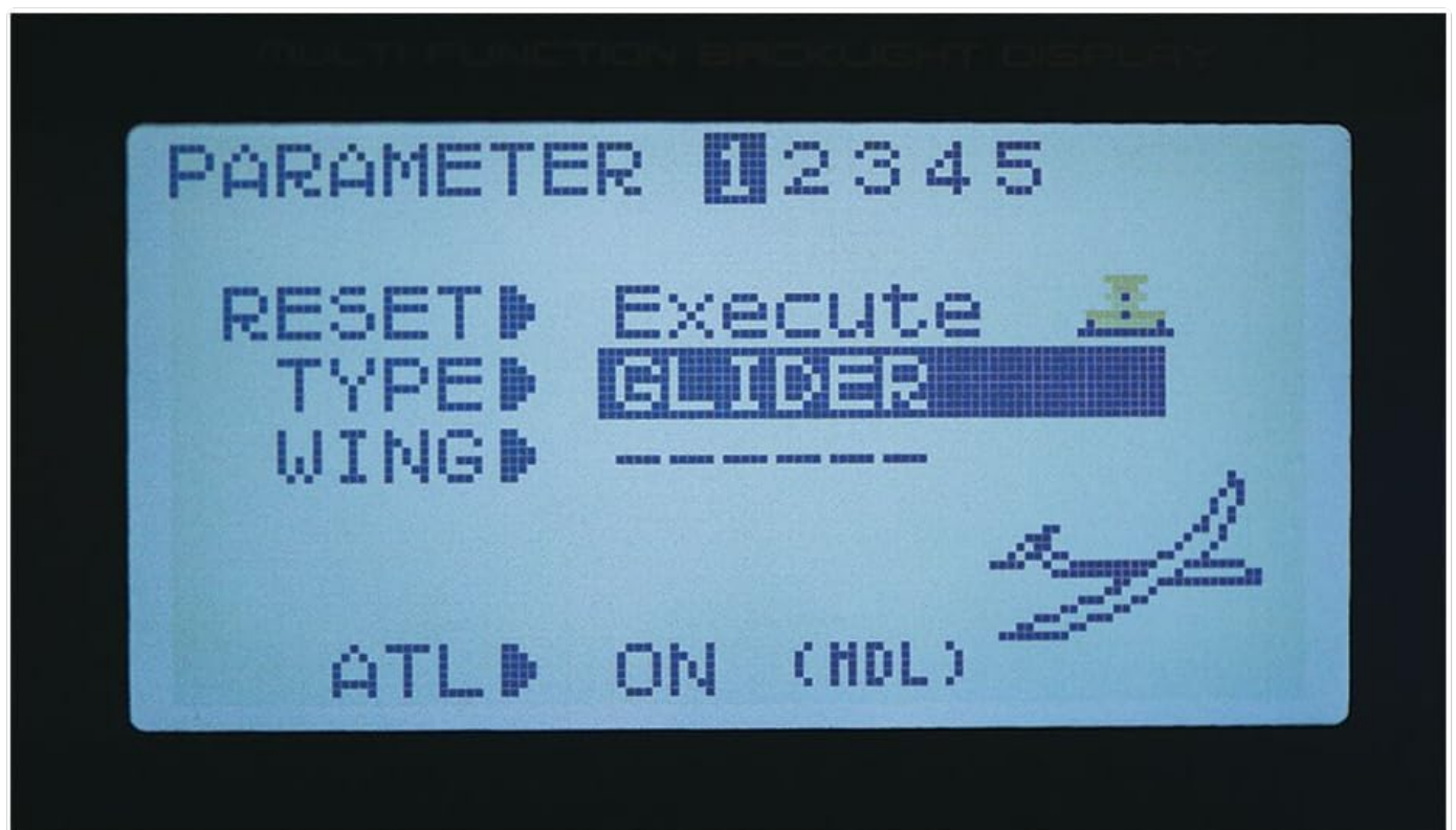
Figure 4: Display showing Glider programming selection.
