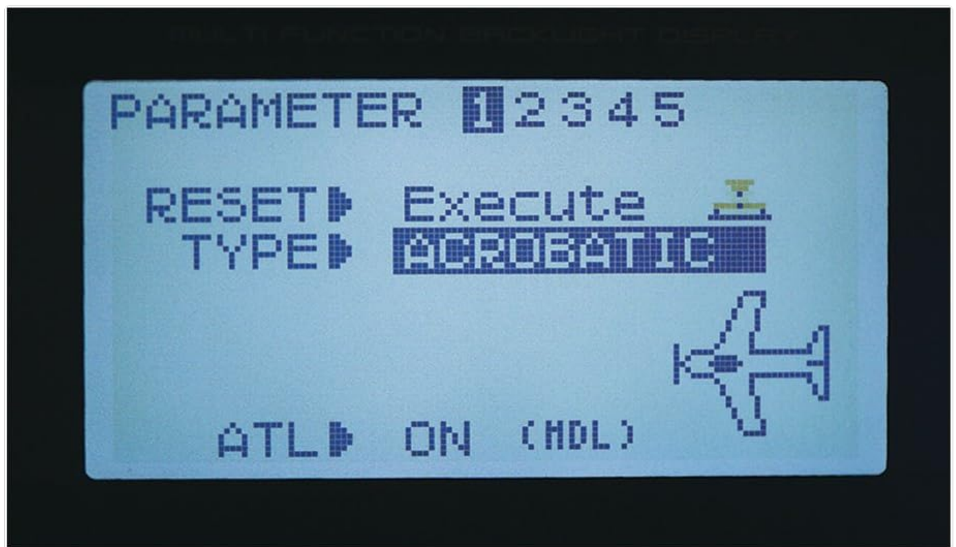
Figure 3: Display showing Airplane (Acrobatic) programming selection.
