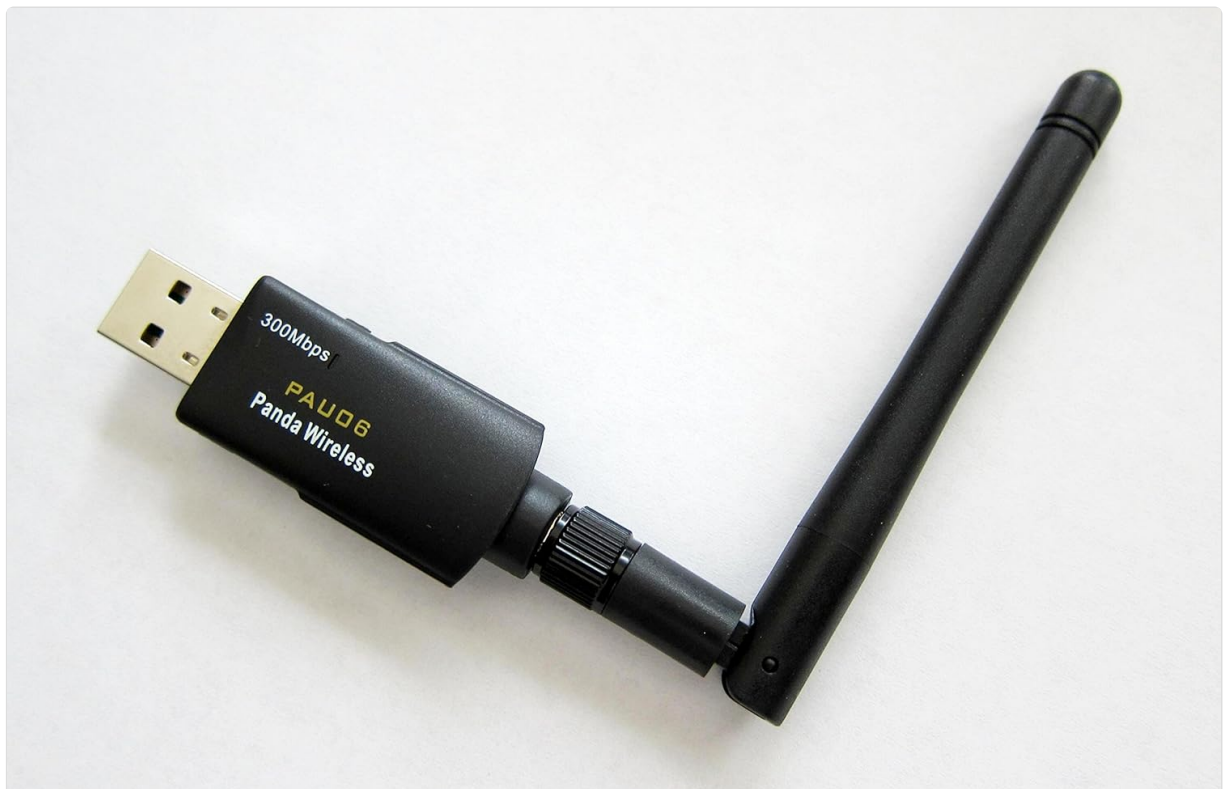
Image: The Panda Wireless PAU06 USB Adapter, showing the USB connector and the adjustable high-gain antenna.
