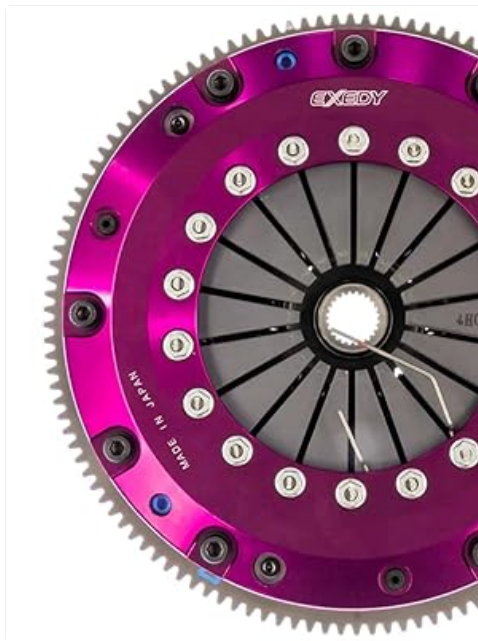
Figure 6.1: Example of an EXEDY clutch and flywheel assembly, illustrating related components.
