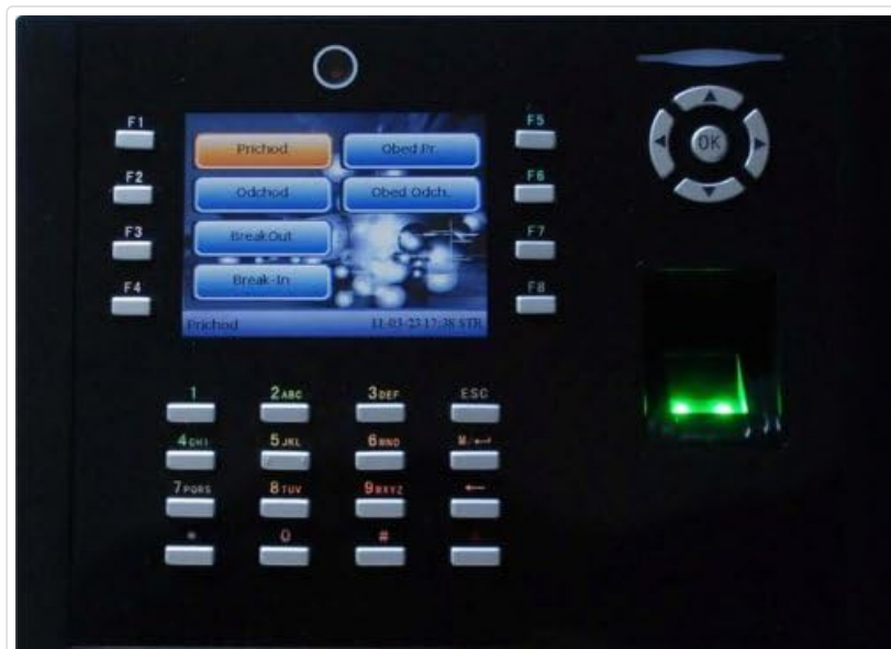
Figure 4: The iClock-360 display showing typical attendance menu options such as 'Prichod' (Clock In), 'Odchod' (Clock Out), 'Break Out', and 'Break In', accessible via the function keys.
