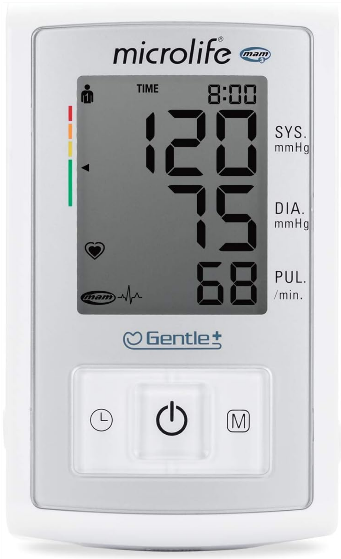
Image: Close-up of the Microlife BP A3 PLUS monitor's digital display, showing time, systolic, diastolic, and pulse readings, along with the MAM and Gentle+ indicators.
