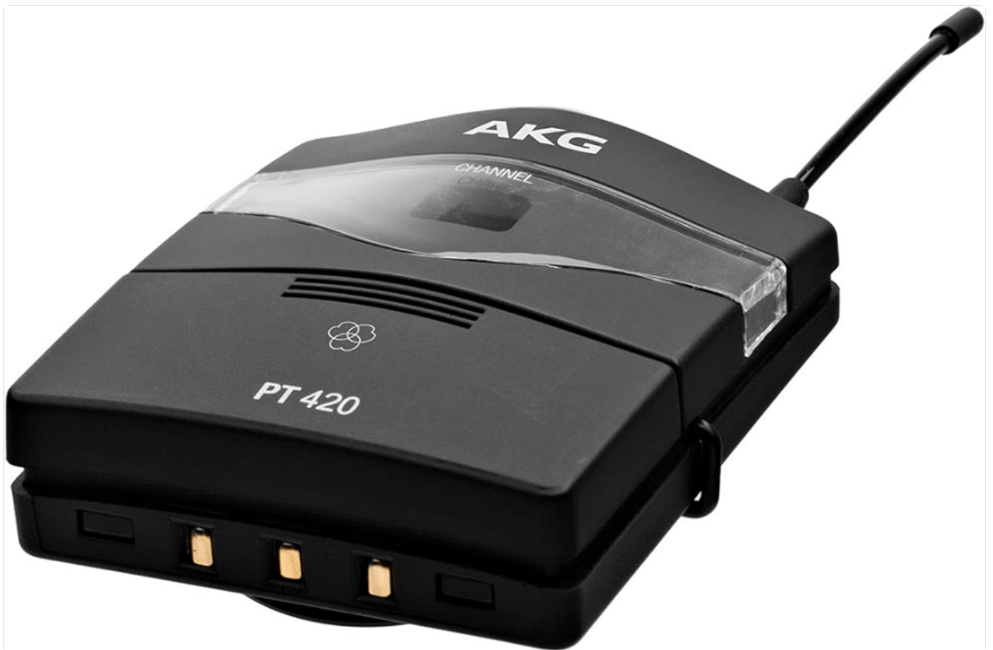
Image: Front view of the AKG PT 420 Body-Pack Transmitter, showing the channel display and battery status indicator.
