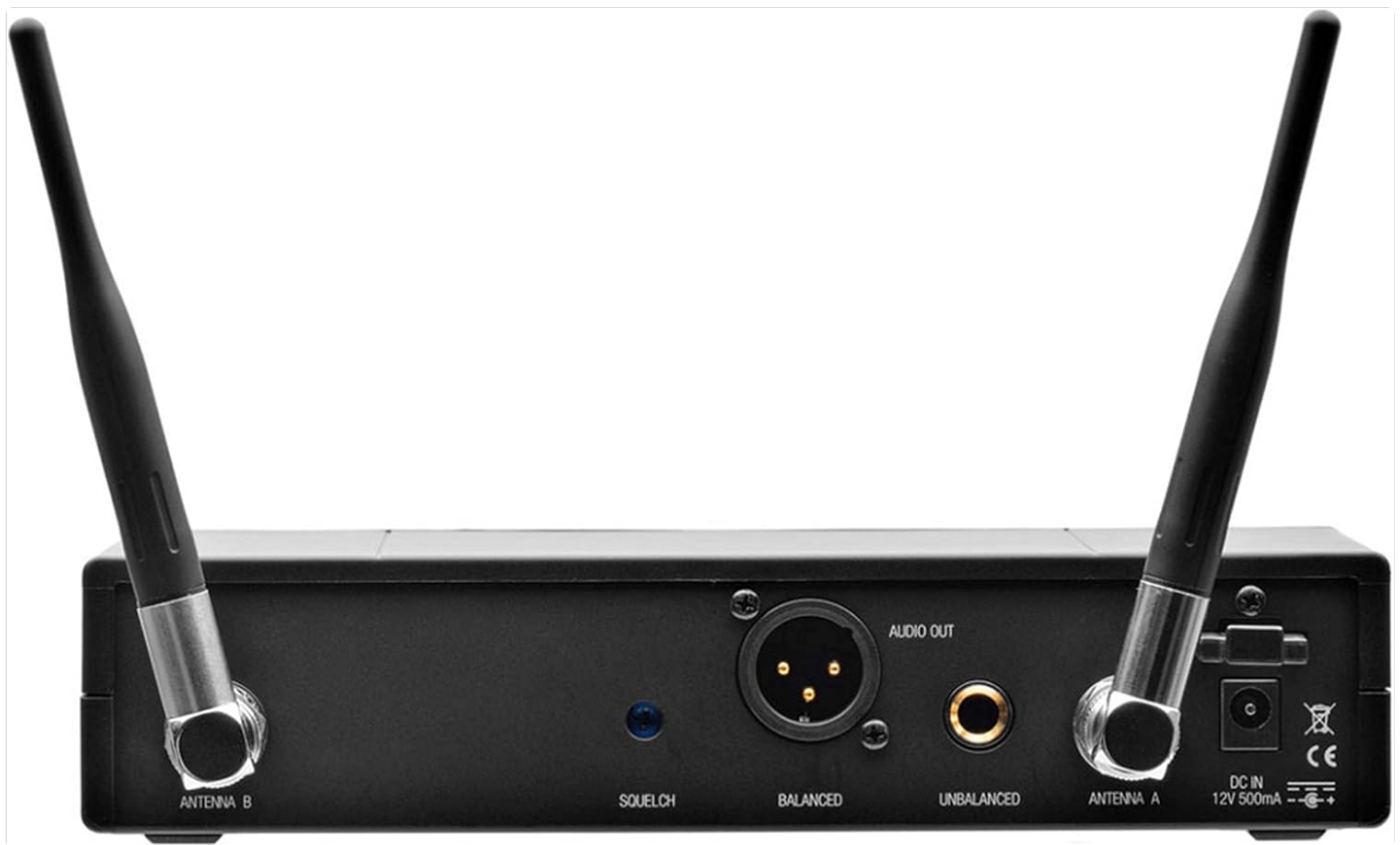
Image: Rear view of the AKG SR 420 Stationary Receiver, showing ANTENNA A and B connectors, SQUELCH control, BALANCED XLR output, UNBALANCED 1/4" output, and DC IN power jack.
