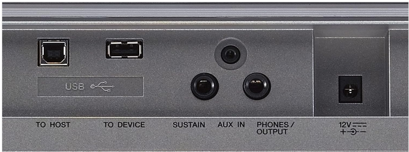
Figure 6.2: Close-up view of the USB TO HOST and USB TO DEVICE ports for computer and storage connectivity.
