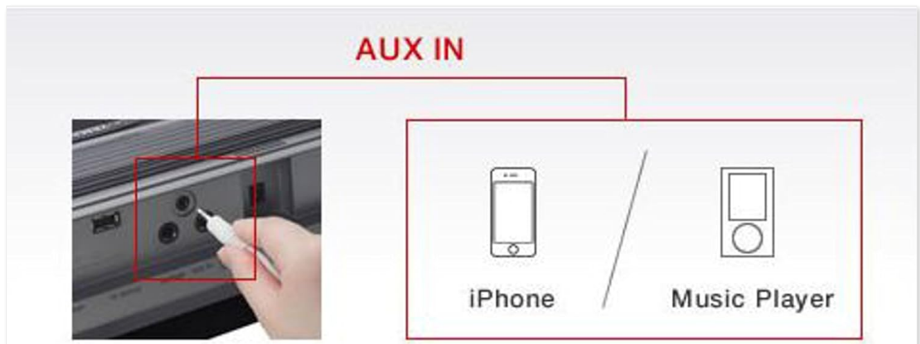
Figure 6.1: Connecting an external audio device to the AUX IN terminal.
