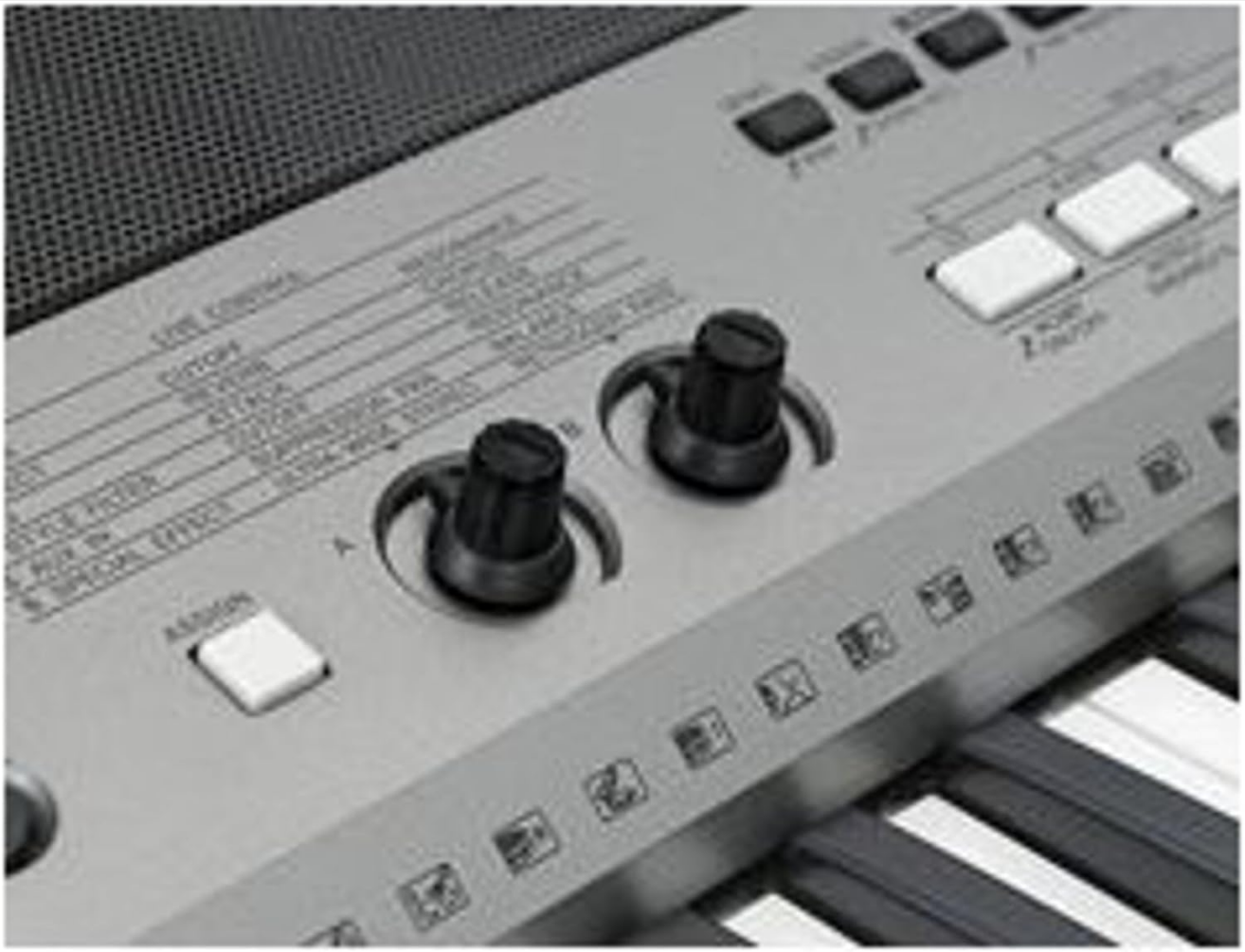
Figure 5.1: Real-time control knobs (A and B) and the ASSIGN button for dynamic sound manipulation.
