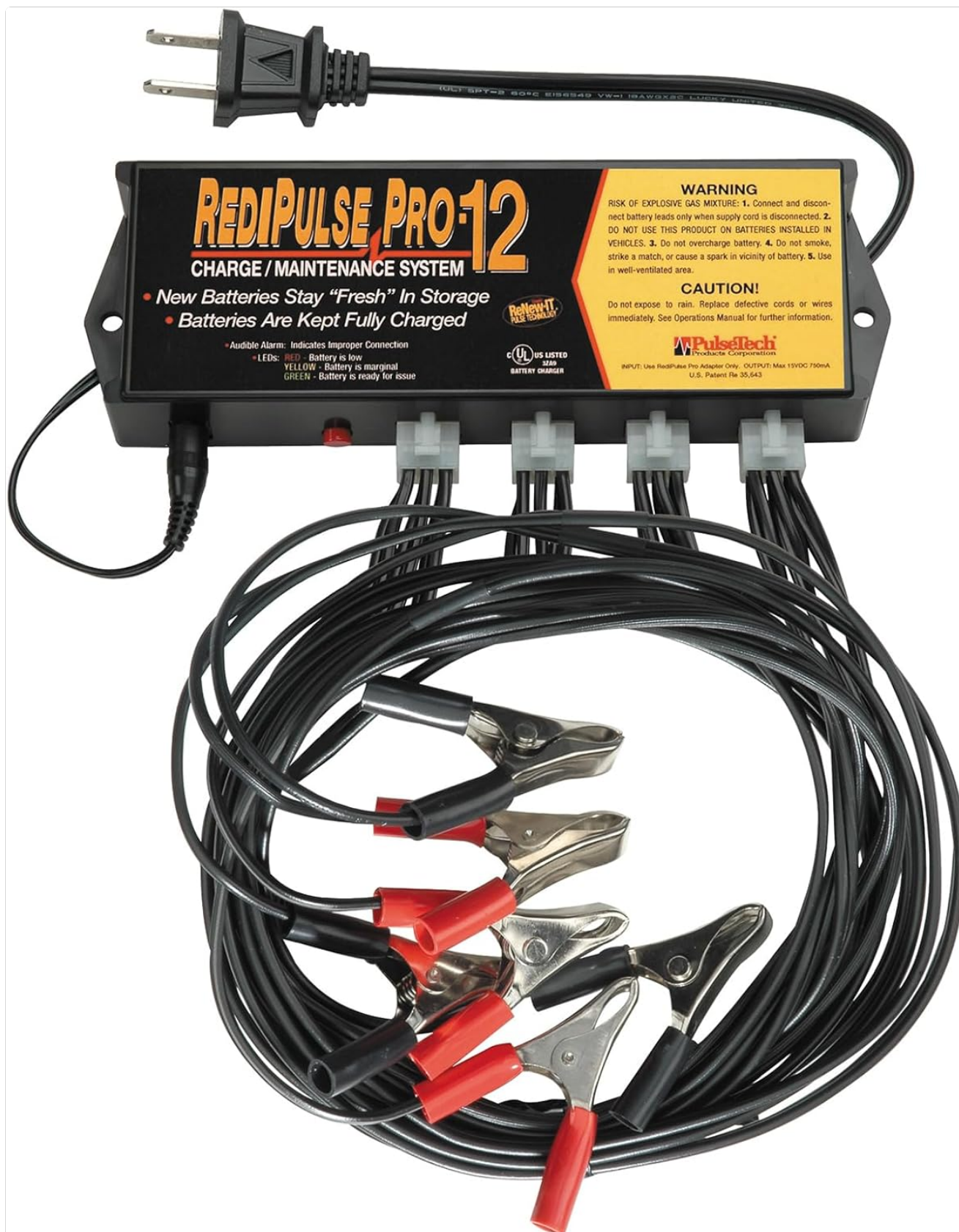
Figure 1: The PulseTech PRO-12-RP RediPulse12 Battery Maintenance System, showing the main unit with multiple battery leads connected.
