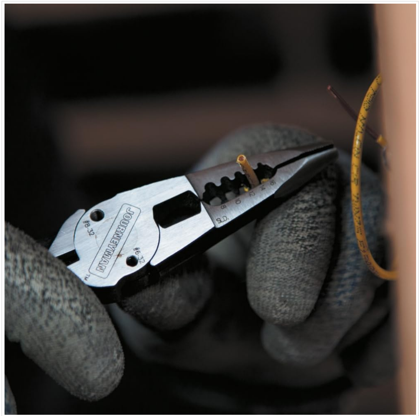
Image: Close-up of the pliers being used to strip wire insulation.
