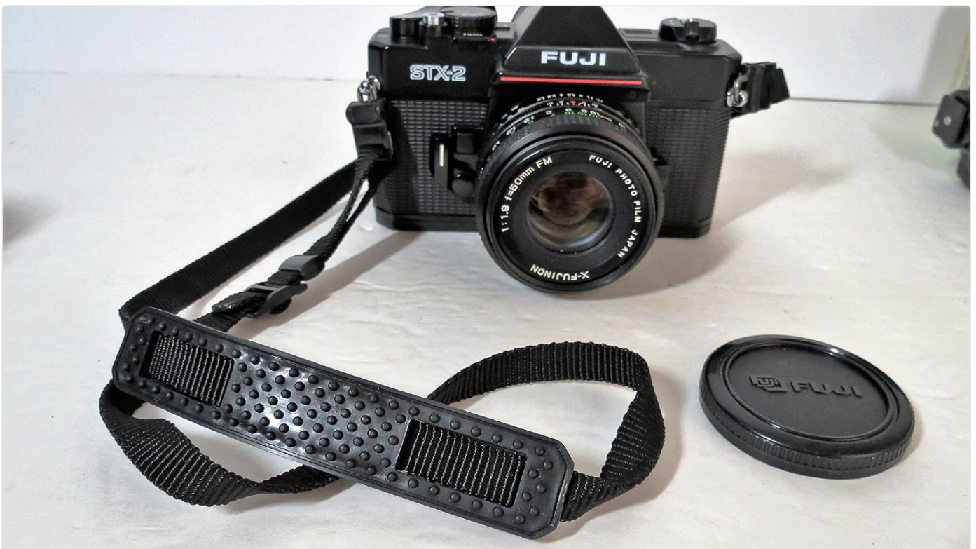
Figure 3.2: Front view of the Fuji STX-2 camera with the lens attached, showing the lens release button and self-timer.
