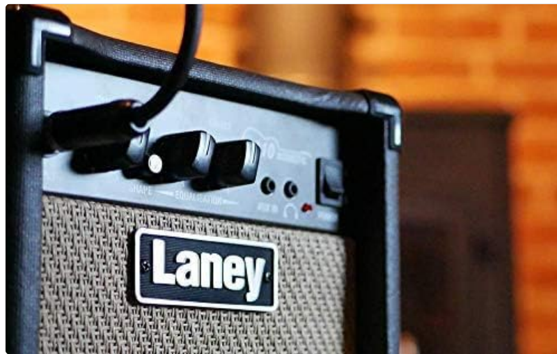
Figure 3: Close-up of the LA10 control panel, highlighting the Volume, Bass, Treble, Shape, Aux In, and Headphone controls.
