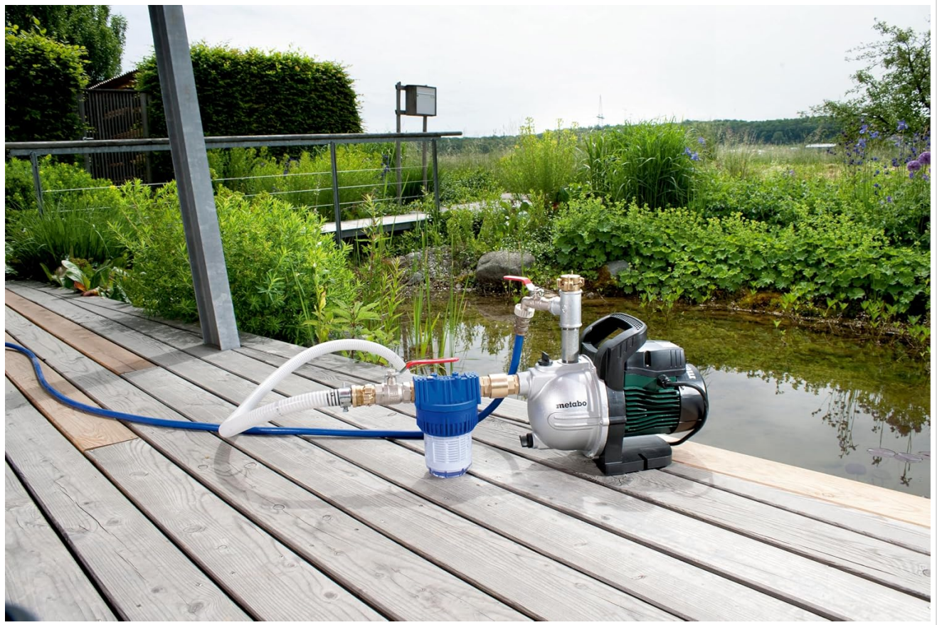
Figure 3.3: The Metabo Garden Pump P 4000 G set up for garden irrigation, demonstrating typical hose connections.
