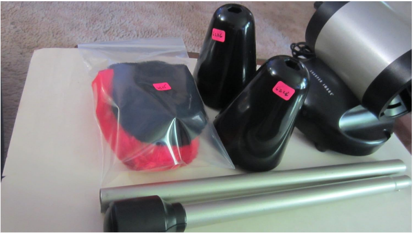
Figure 2.1: Overview of the Sharper Image Shoe Polisher CA825, showing the main unit, two black polishing brushes, a plastic bag containing red and black buffing pads, and two silver extension poles.
