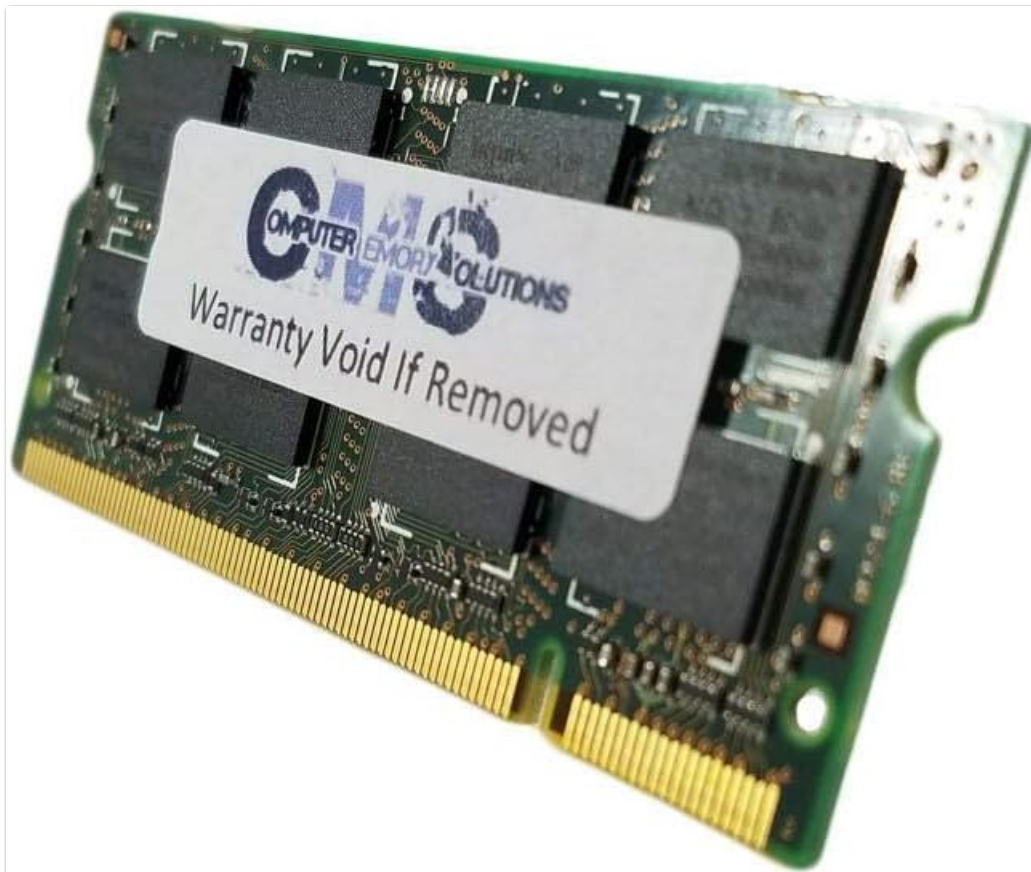
Figure 2: Angled view of the CMS 2GB DDR2 SODIMM memory module, showing the gold connectors.
