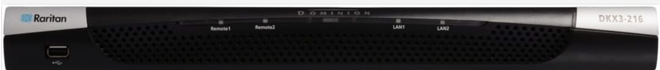
Figure 1: Front Panel View. This image displays the front panel of the Raritan Dominion KX III DKX3-216 KVM-over-IP Switch, showing the Raritan logo, Dominion branding, model number DKX3-216, and indicators for Remote1, Remote2, LAN1, and LAN2. A USB port is visible on the left side.
