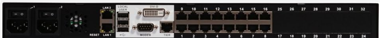
Figure 2: Rear Panel View. This image shows the rear panel of the Raritan Dominion KX III DKX3-216 KVM-over-IP Switch, highlighting the dual power inputs, LAN ports (LAN1, LAN2), a reset button, local user ports (USB, DVI-D, VGA, Serial), and 16 KVM ports numbered 1 through 16.
