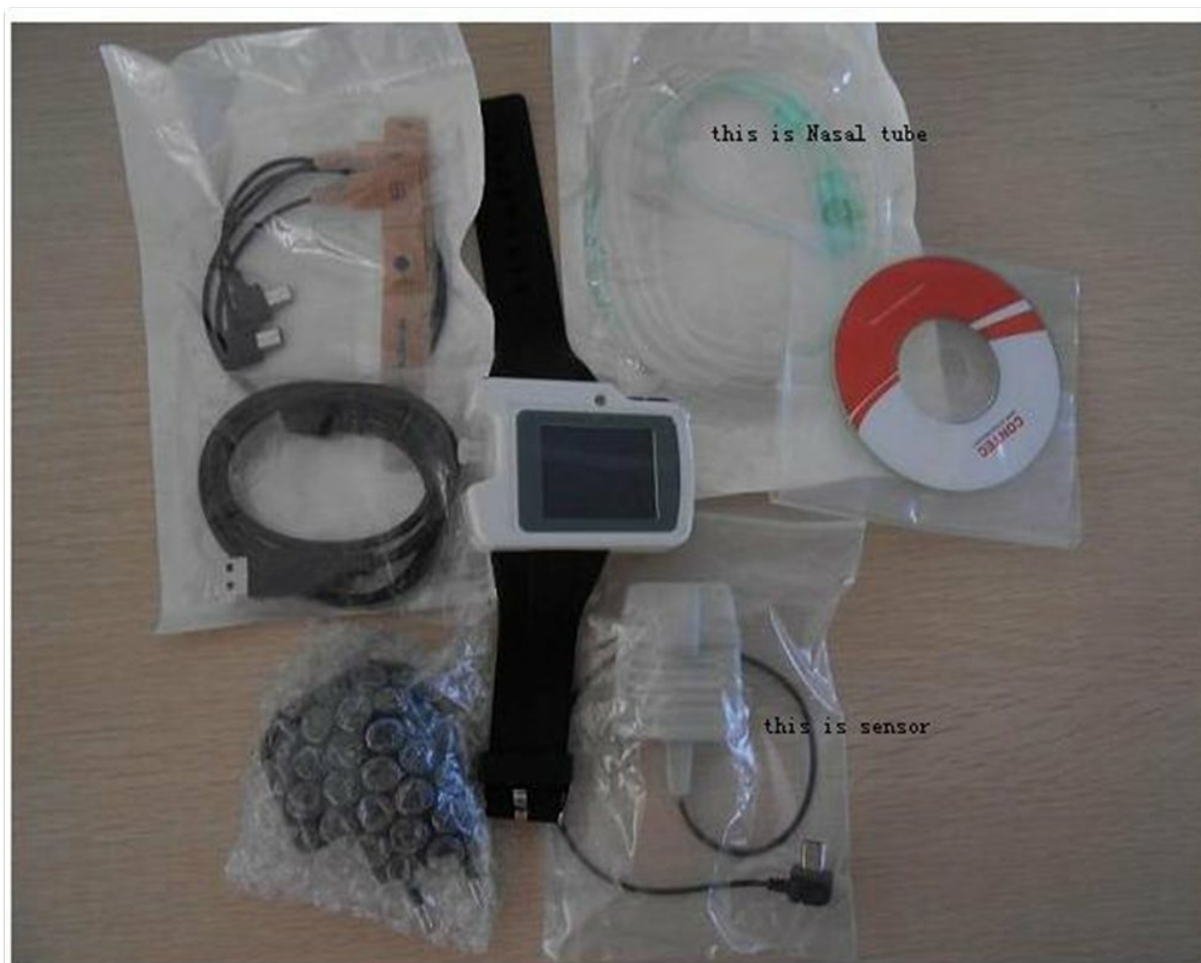
Figure 2: An overview of the items typically included in the CONTEC RS01 product package. This includes the main unit, nasal tube, sensor, and various cables.
