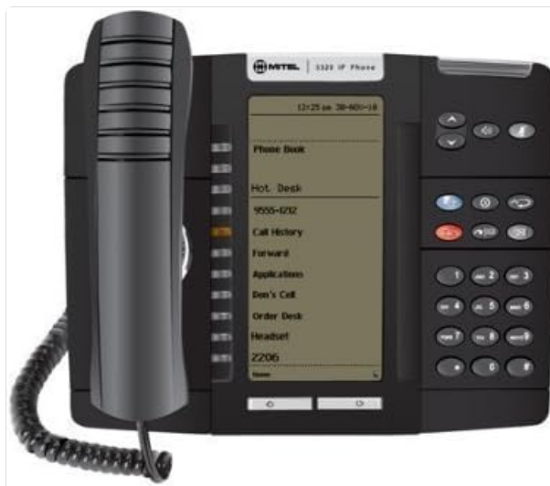
Figure 1: The Mitel 5320e IP Phone. This image displays the phone's main components including the handset, the backlit LCD screen showing "Phone Book" and other menu options, and the numeric keypad along with various function buttons.
