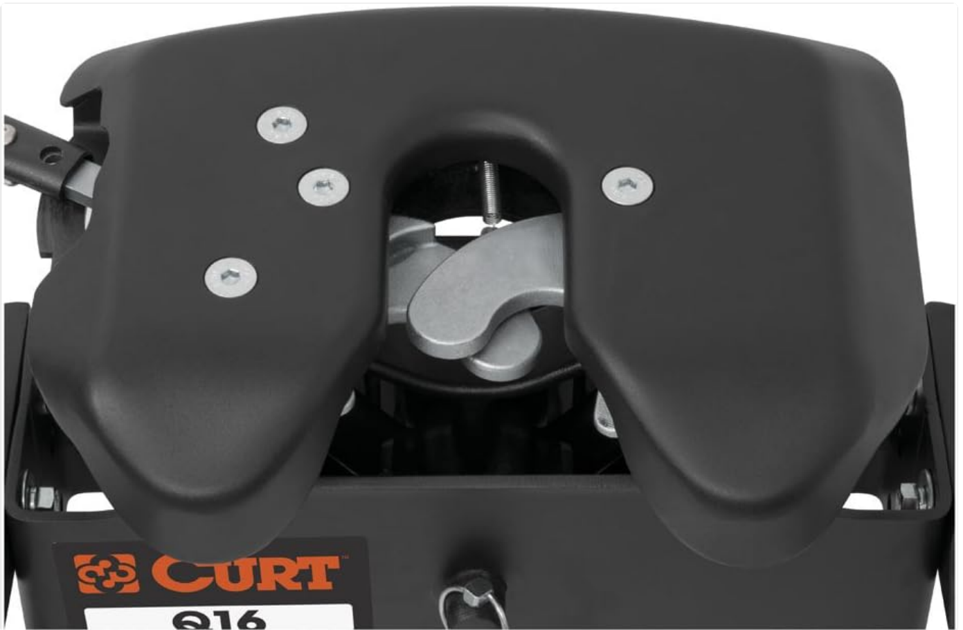
Image: The hitch head with jaws open, prepared to receive the trailer's kingpin.
