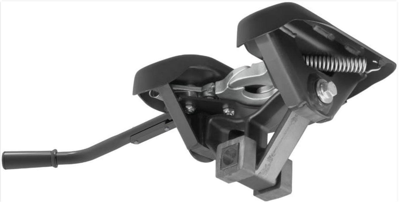
Image: The lockable handle of the CURT A16 5th Wheel Hitch in the uncoupled position.
