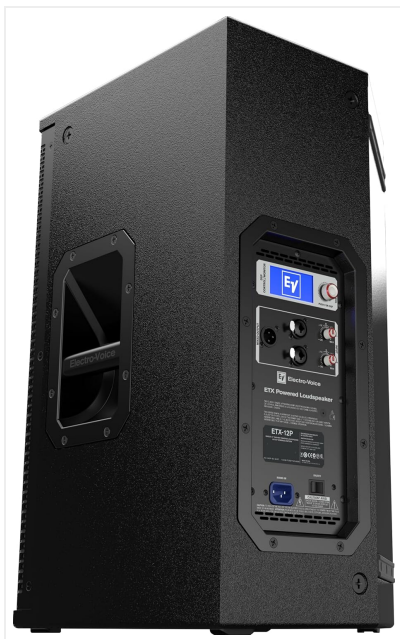
Figure 3.3: Rear Panel. This image details the rear control panel of the ETX-12P, including input/output connectors (XLR), the power switch, AC inlet, and the LCD screen with the single-knob DSP control. This is where all audio and power connections are made and where sound parameters are adjusted.
