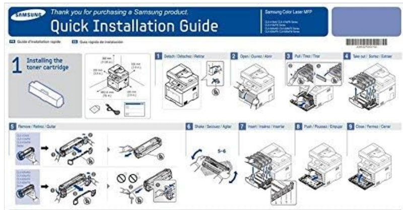
Figure 3: Excerpt from the Quick Installation Guide showing toner cartridge installation.
