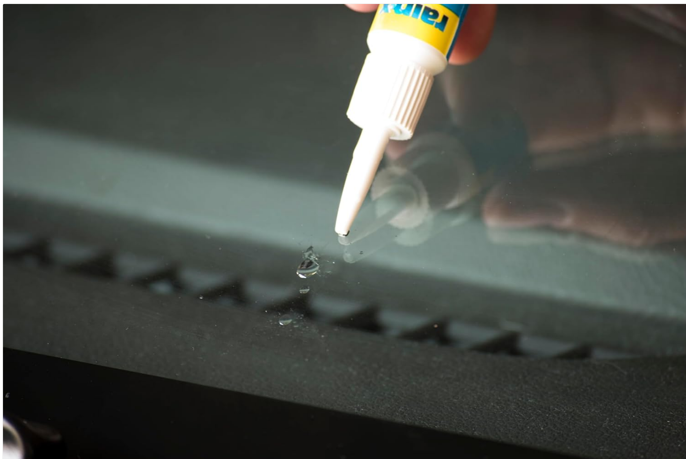
Detailed view of the resin application process on a windshield chip.
