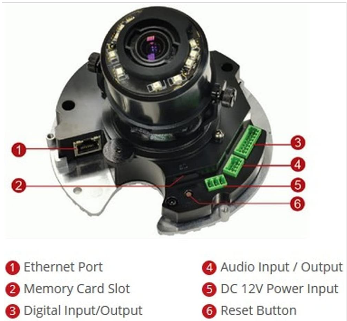
Figure 2: Internal view of the ACTi B61 camera with key components labeled.
