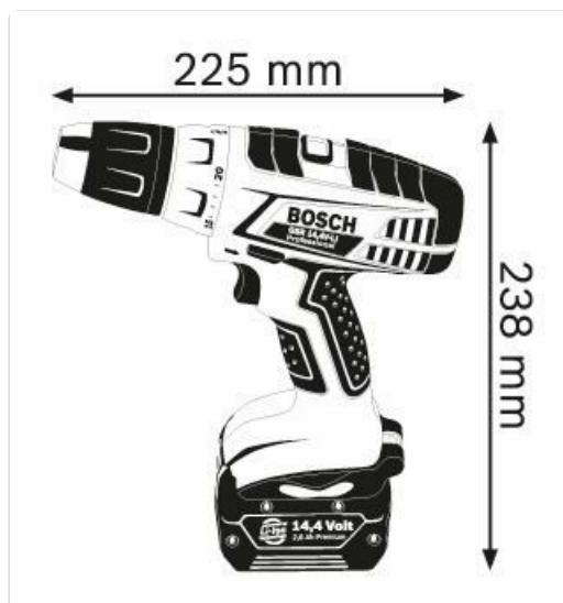
Figure 3: A technical diagram illustrating the dimensions of the Bosch GSR 14.4 VLi drill driver, showing its length (225 mm) and height (238 mm). This provides a clear understanding of the tool's physical size.
