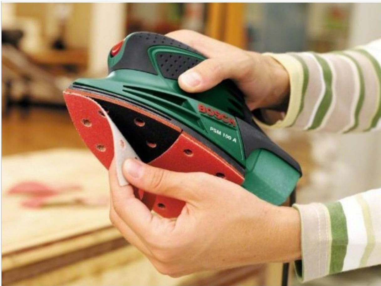
Figure 2: Attaching a sanding sheet. This image shows hands pressing a red, triangular sanding sheet onto the black sanding plate of the tool, demonstrating the hook-and-loop attachment method.
