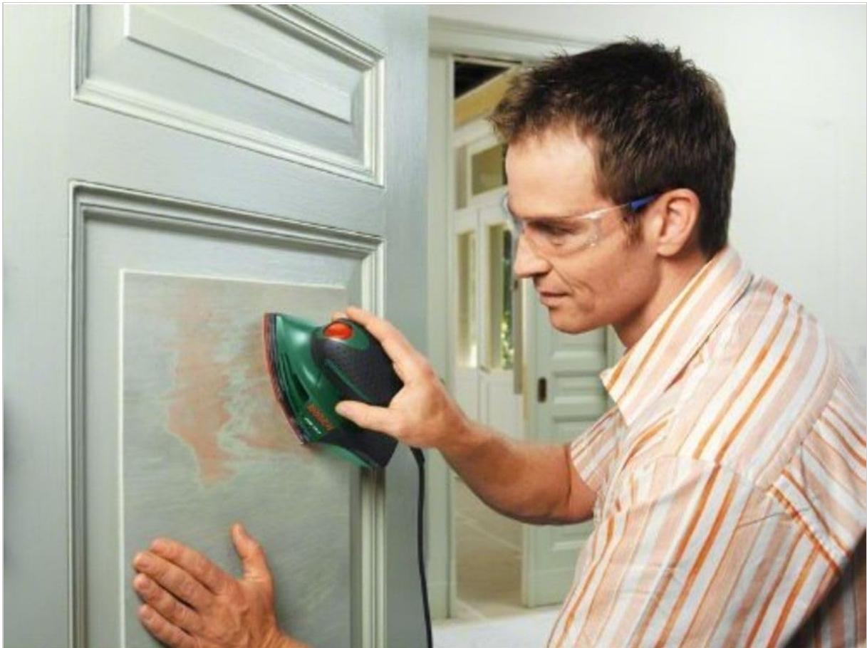
Figure 4: Sanding a door panel. A person is using the sander on a door panel, illustrating its suitability for preparing painted or varnished surfaces.
