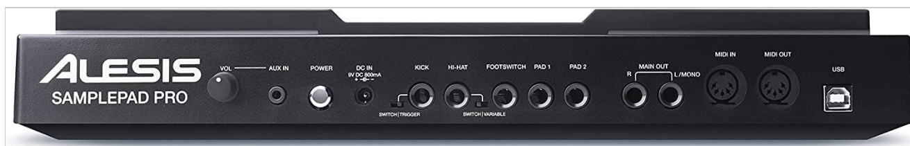
Figure 2: Rear panel connections of the Alesis SamplePad Pro.
