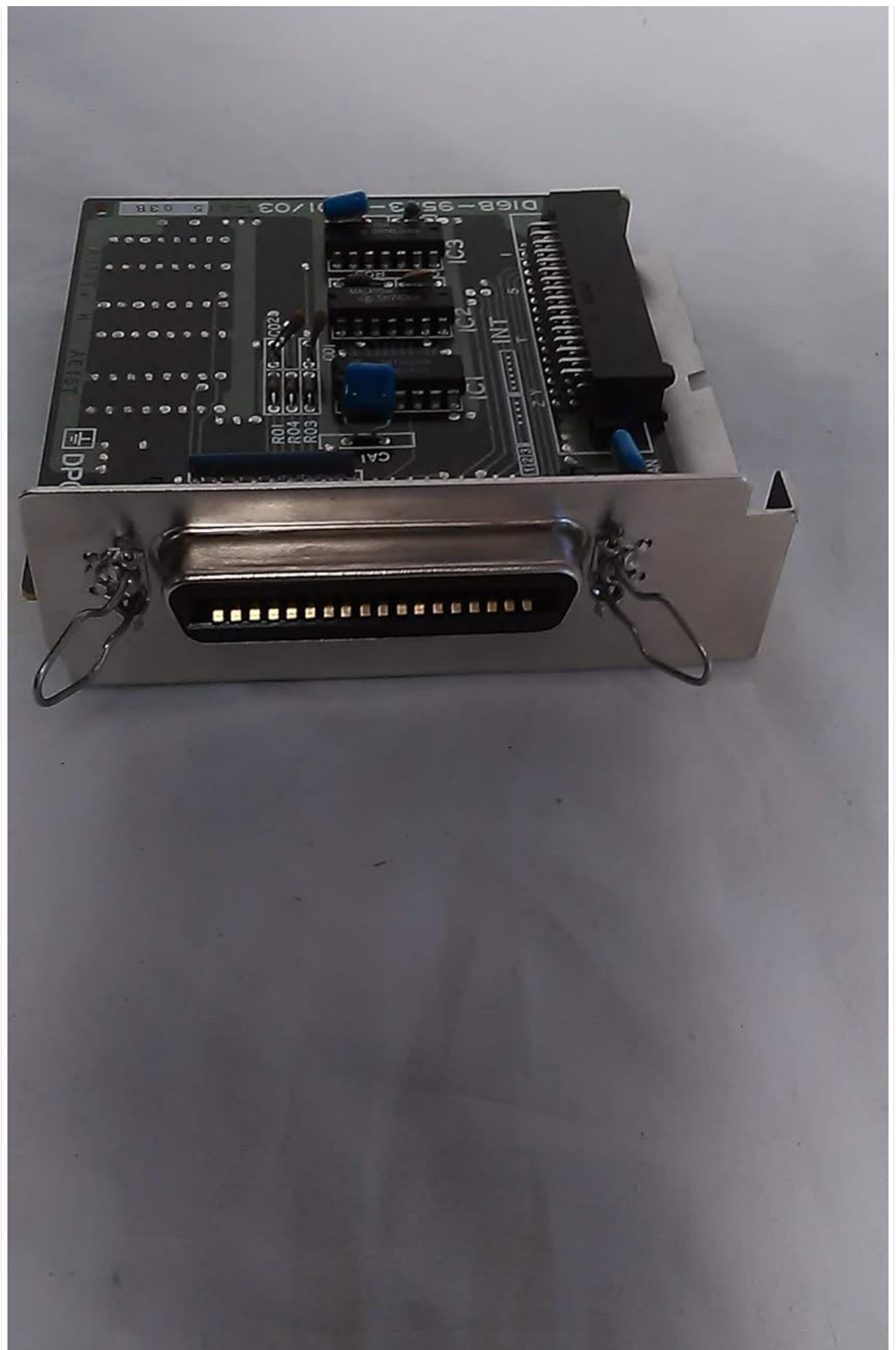
Figure 3: Close-up view of the Centronics parallel port connector on the Fujitsu S26361-F2814-V8 card. This is the external interface for connecting compatible peripherals.
