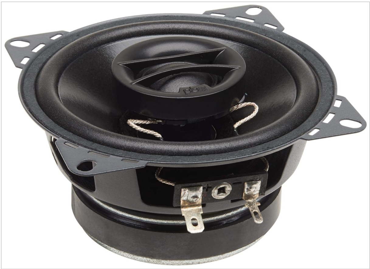
Image: Side view of a Powerbass S-4002 speaker. This view highlights the speaker's magnet, the sturdy metal basket, and the two spade terminals for electrical connection.
