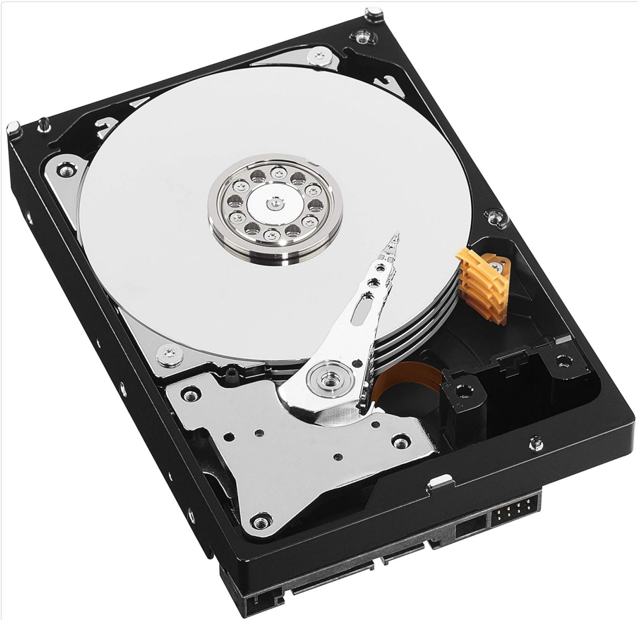
Figure 3.1: Angled view of the WD Purple hard drive, highlighting the SATA power and data connectors for system integration.
