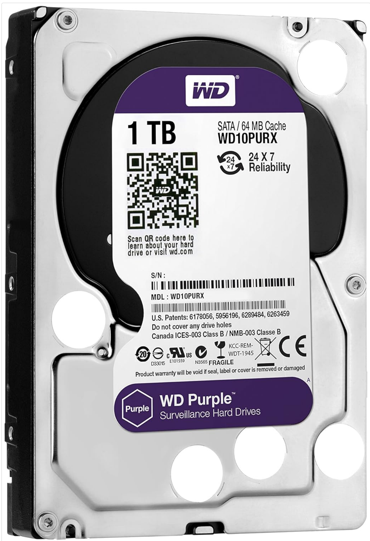
Figure 3.2: Back label of the WD Purple drive, displaying the model number WD10PURX and a QR code linking to WD Purple product information .
